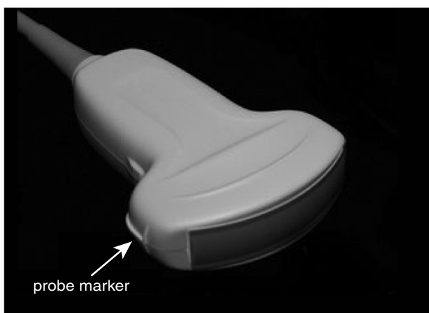
Fig. 1. Low frequency (2–5 MHz) curvilinear probe.
